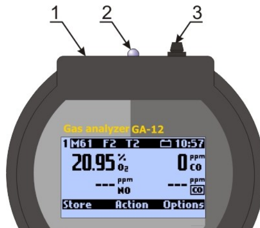
Drawing 1. Analyser's connection in the top part of the housing.
